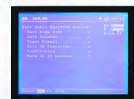
Display (Graphic LCD 320 x 240 Dots)
